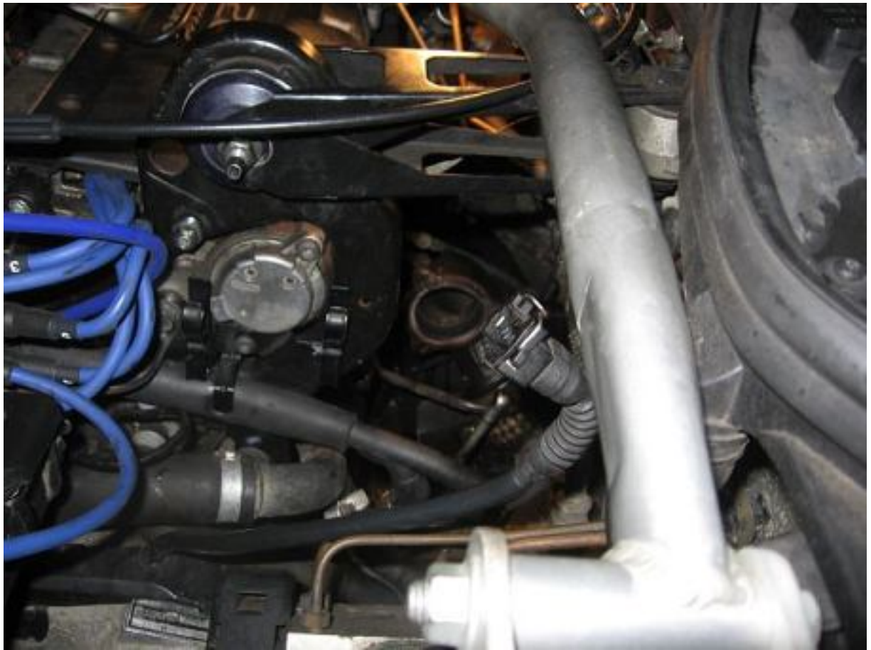
There's the original turbo, as it was removed. See what I mean about the coolant pipe and its inaccessible banjo bolt :-)
