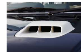
Inter cooler vent
