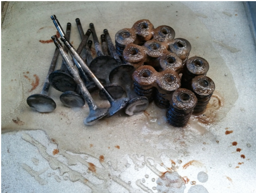
Valves and springs now soaking
