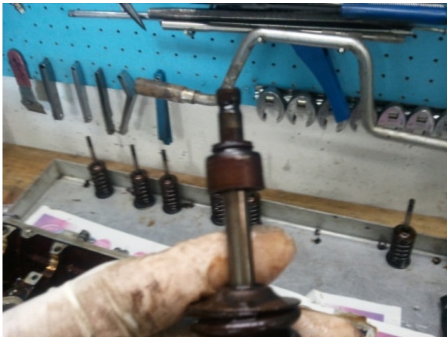
The old seal nearly slides down the valve on its own
