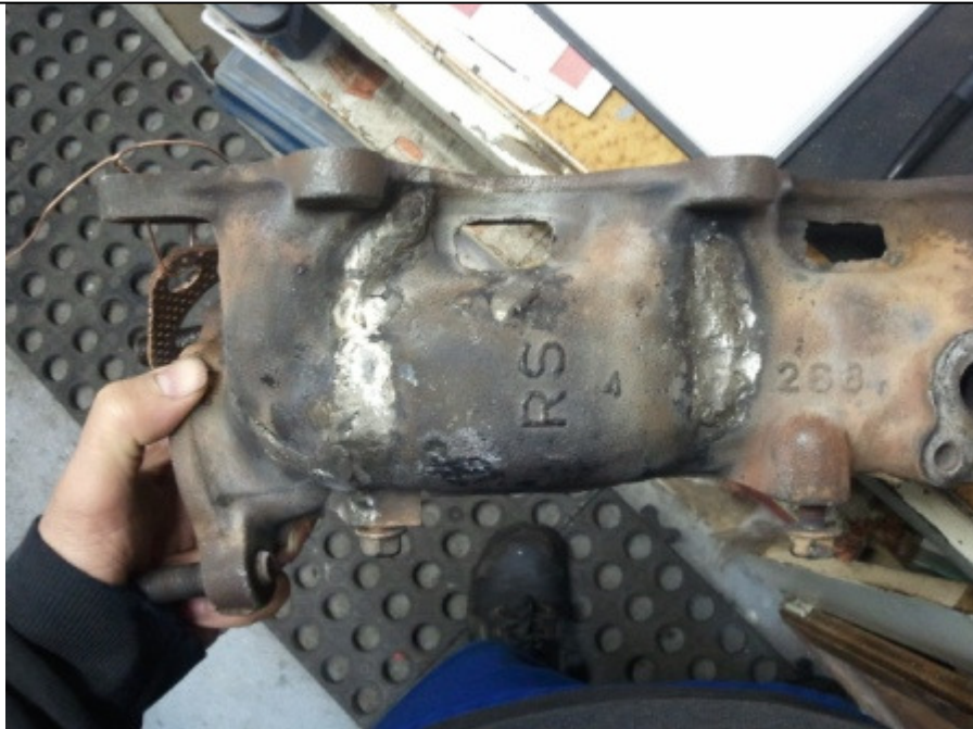
Tempory measure until I decide on branches or a new manifold
