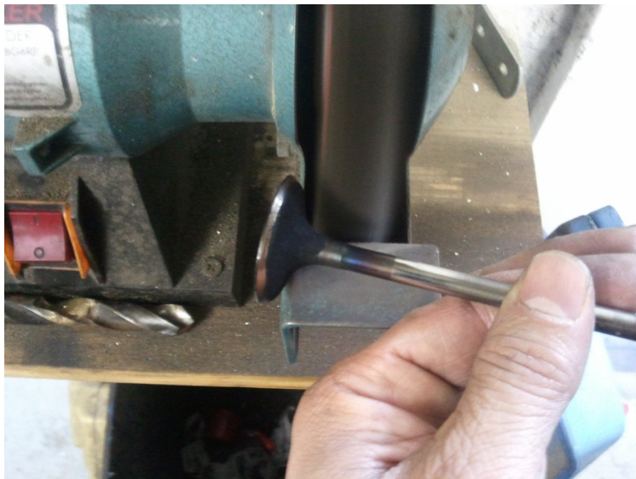
Clean stubborn carbon off the valves with a wire wheel
