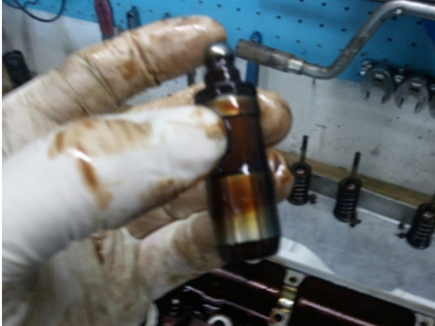
This is a hydraulic lifter or lash adjuster
