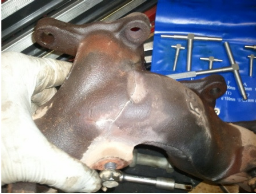
My exhaust manifold was also cracked
