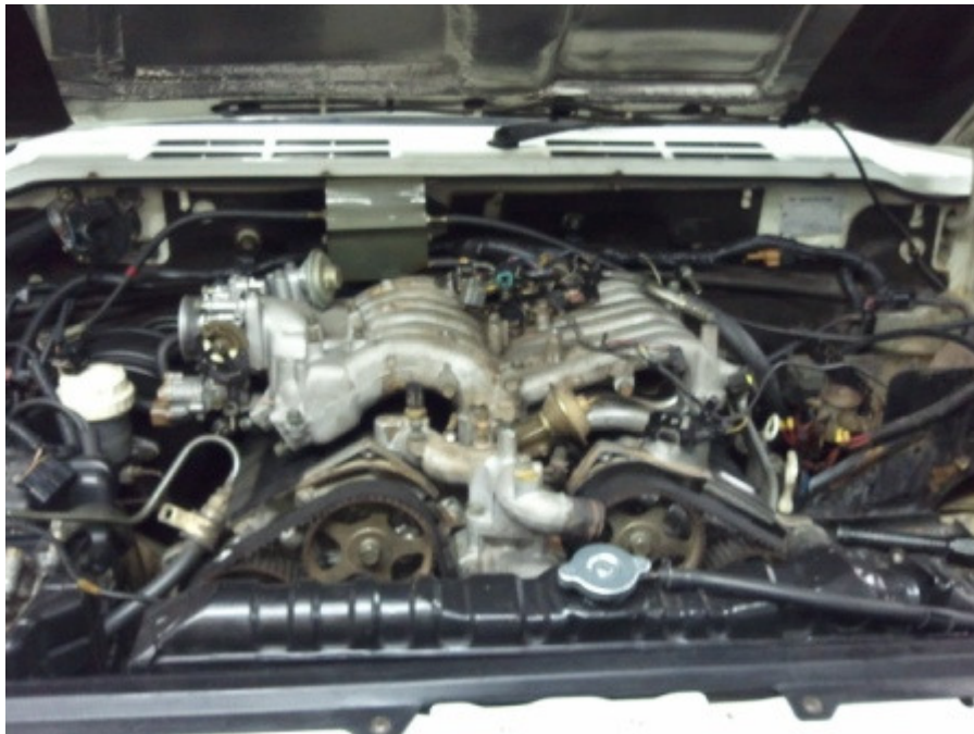
Manifold now on
