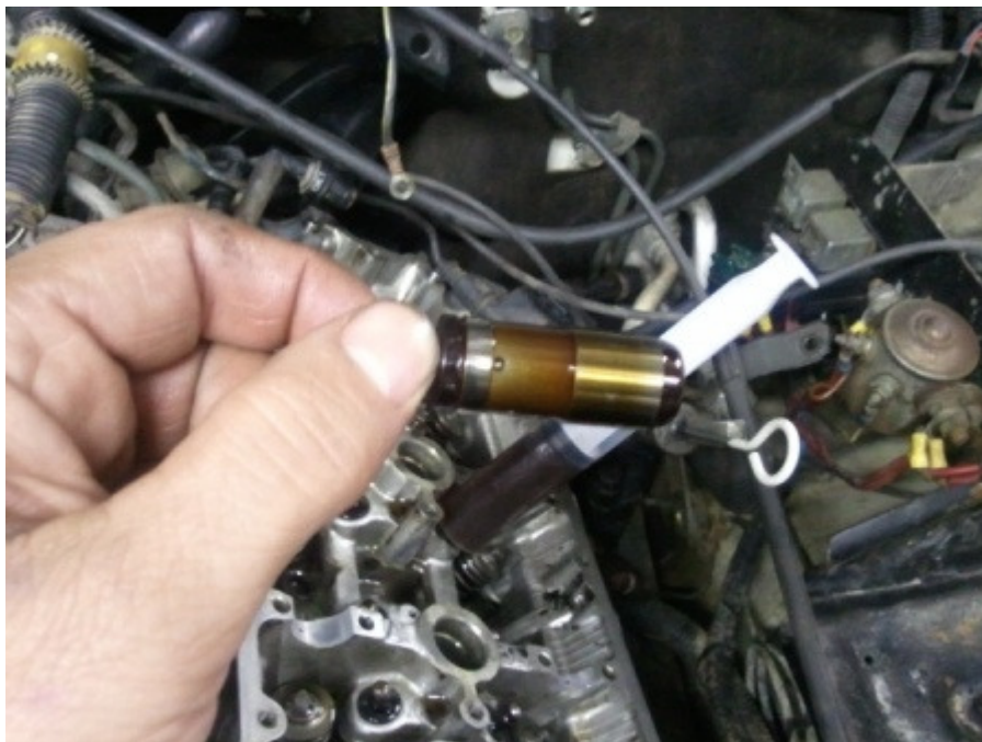
To prime the hydraulic lifter I used a syringe and needle with the lifter in the upright position, do not force the needle into the lifter if you use this method
