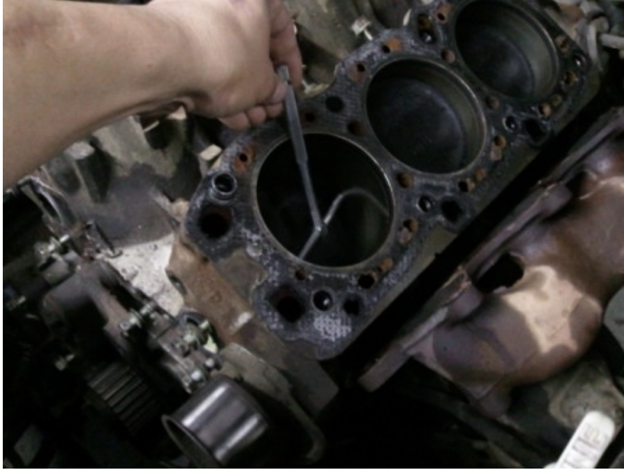
A quick check of the bores before cleaning starts
