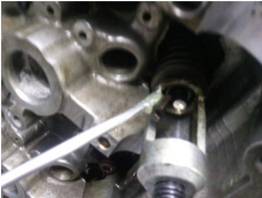
The trick here is to use a long thin screw driver with just the right amount of magnetism and grease
