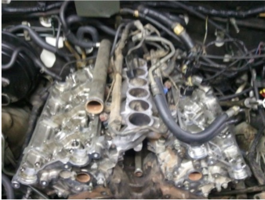
Bottom half of inlet manifold and fuel injection rail now on
