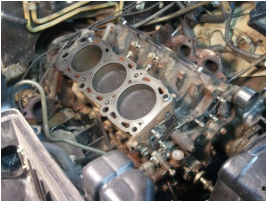
Mating surface now cleaned with emery paper and thinners
