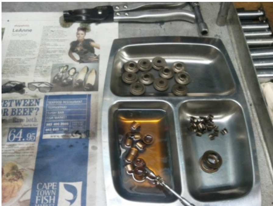
Try to place your components in a methodical order so as not to forget something like a valve spring seat
