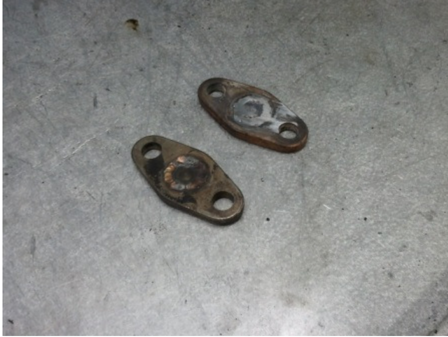
This was my old exhaust gas recirculation pipe which I cut up and welded close to make blanking off caps hot exhaust gas in the inlet manifold can't be good for performance in my view
