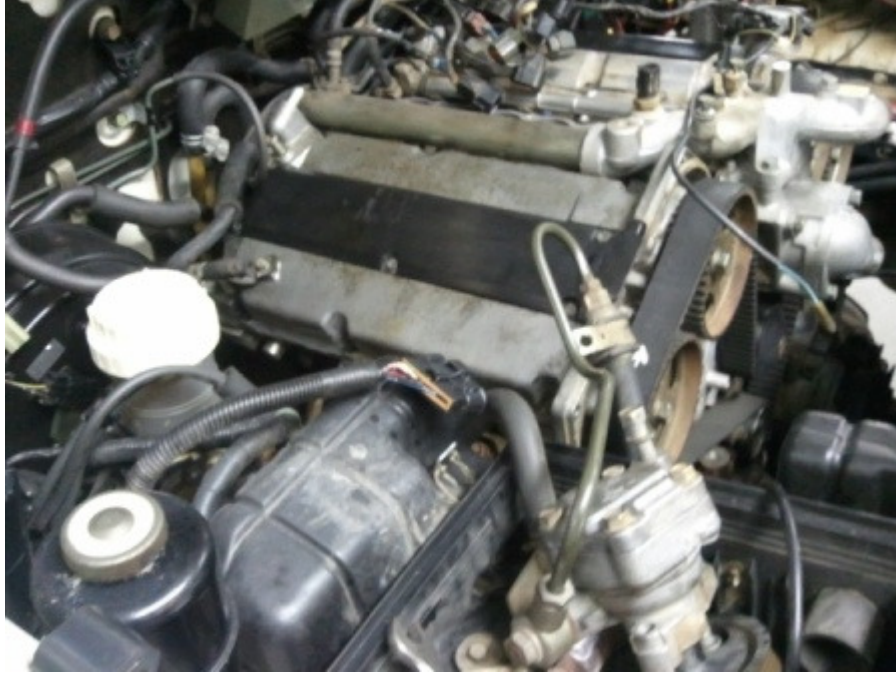
Thermostat housing on and all plumbing connected
