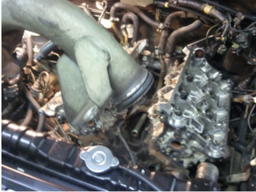
Water cross over from front to back replace this o ring
