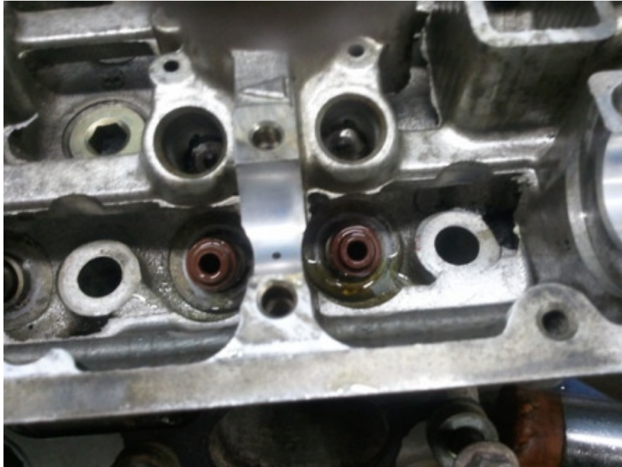
New valve seals in place
