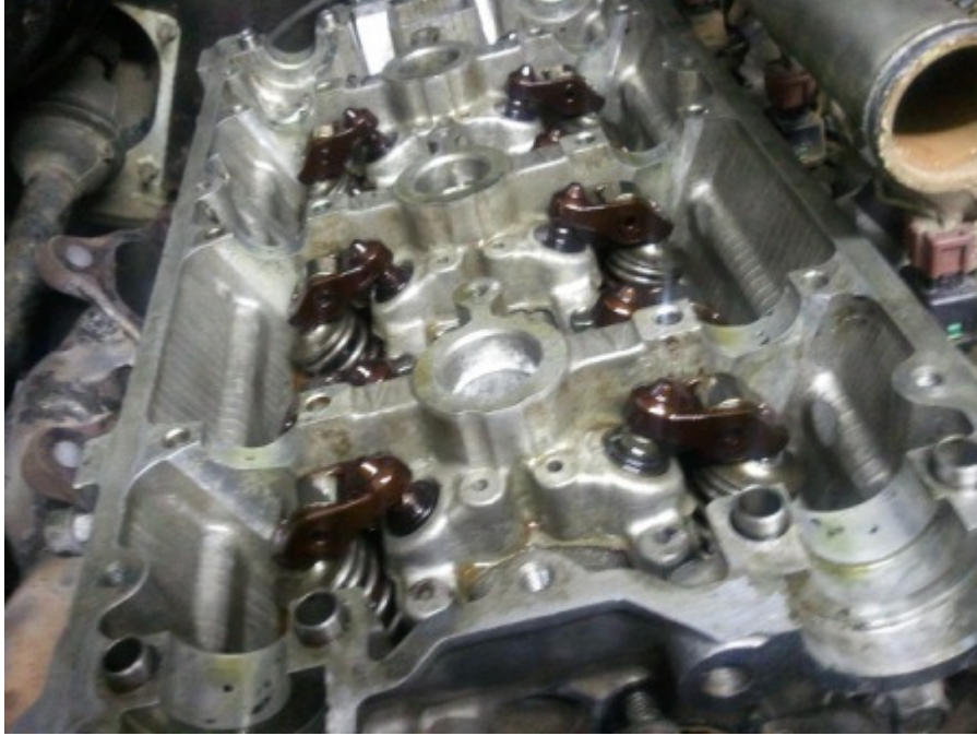
Rockers now in place
