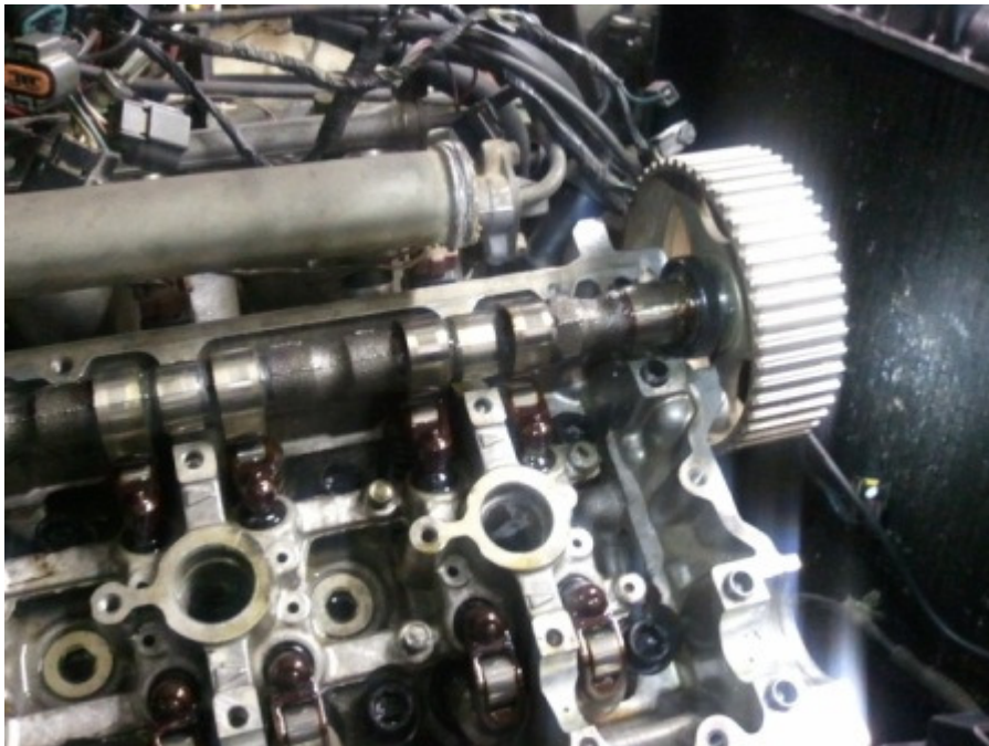
First cam being installed
