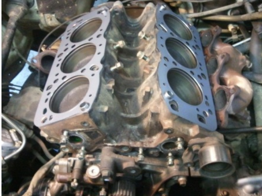
New head gaskets in place
