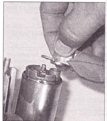
4.6b Detach the inlet strainer from the fuel pump
